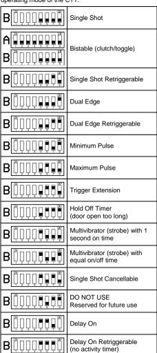
**Note:** All the timing diagrams shown are for a positive trigger and fail secure relay (Dip switches 1 and 2 on bank B are off).
